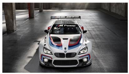
In 2016, the BMW M6 GT3 will replace the BMW Z4 GT3, which has been in action since 2010. The new car is powered by a 4.4-litre V8 engine with M TwinPower Turbo technology, which has been modified for use in motor racing. The power train has dry sump lubrication and generates up to 585 hp — with the whole car weighing less than 1,300 kilograms.
