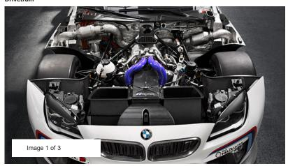
The low position of the power train further lowers the centre of gravity, thus improving performance. The transaxle gearbox ensures weight is distributed perfectly between the front and rear axles.
